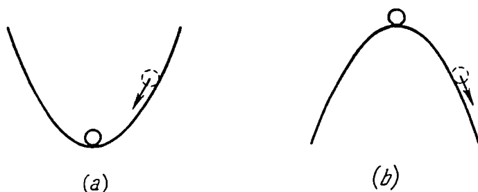
Fig. 16. (a) Stability : after small departures from the equilibrium position (bottom) the marble returns to it: "Small causes have small effects." (b) Instability : small departures originate large effects: "Small causes have large effects."
